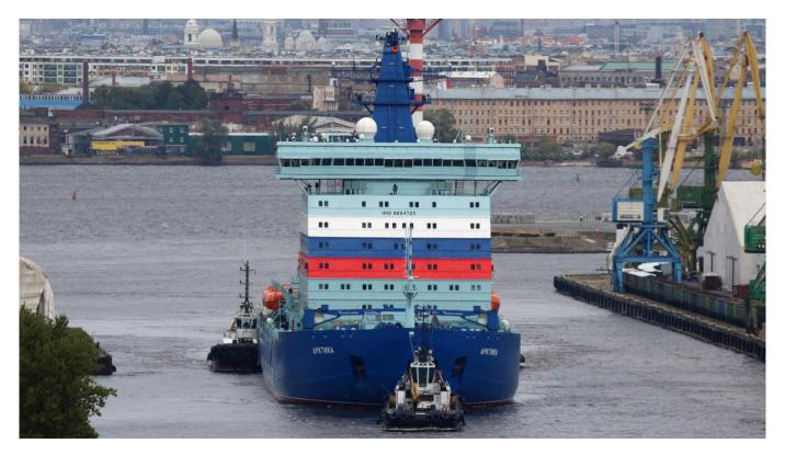
According to its constructors, the Arktika can cut through ice that is 2.8 meters (around 9 feet) thick. **Valentin Egorshin / TASS**
