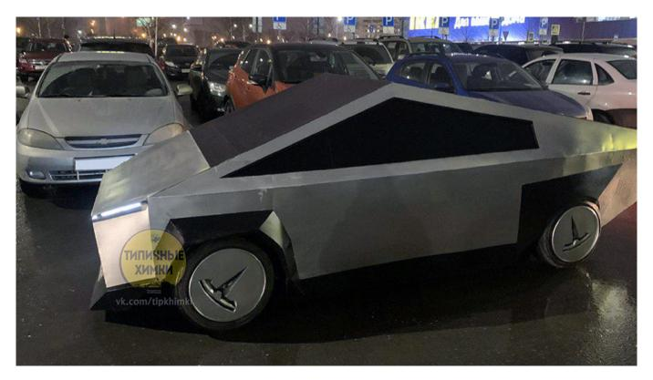
The Cybertruck reproduction is based on Russian automaker AvtoVAZ's popular Lada Samara, a small hatchback that has a similar angular body, but runs on gasoline. **tipkhimki / Vkontakte**
