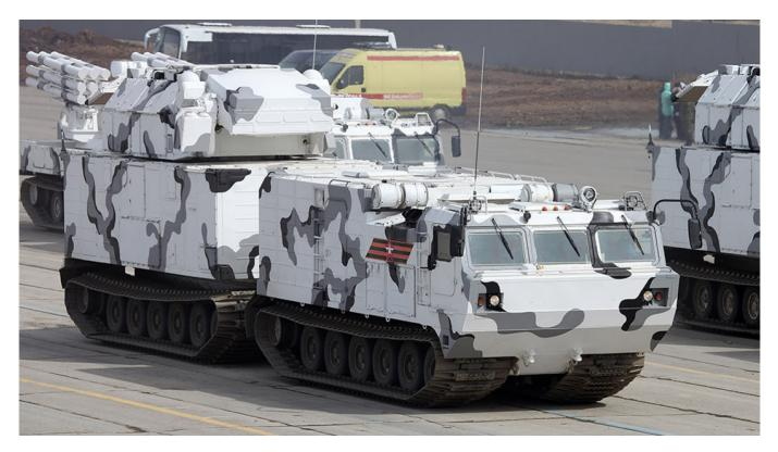
The Tor-M2DT is a variant of the Tor missile system (SA-15 "Gauntlet") that was first introduced in the late 1980s. **Vitaly Kuzmin / Wikicommons**
