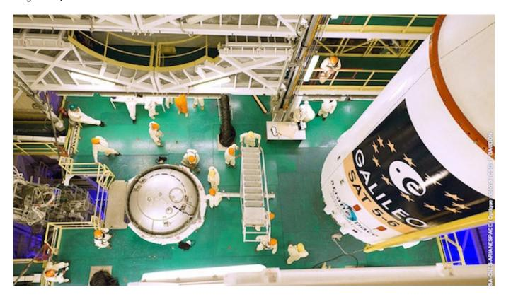
The launch fairing containing the two Galileo satellites and their dispenser atop the Fregat upper stage next to the top of the three-stage Soyuz launcher in the mobile gantry at the launch zone, about to be attached together. Integration occurred on the evening of Aug.19, 2014.
