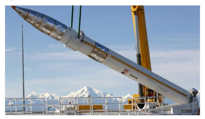
A ground-based missile interceptor is lowered into its missile silo during a emplacement at the Missile Defense Complex at Fort Greely, Alaska.
